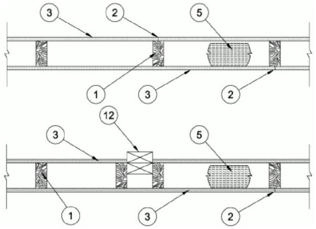
1. Wood Studs - Nom 2 by 4 in. spaced 16 in. OC max, effectively firestopped.
